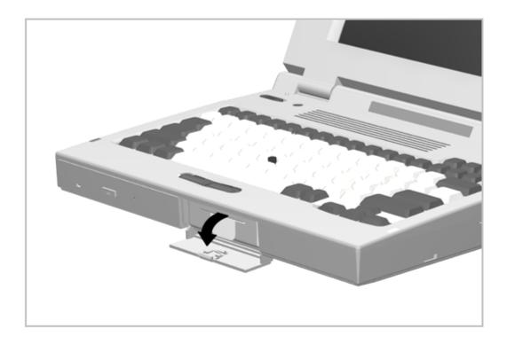
Figure 5-20. Removing the Hard Drive Bay Door
